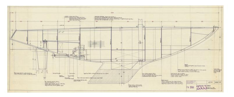
Photo8\_Section plan of Didon III, with the ferrocement hull.
